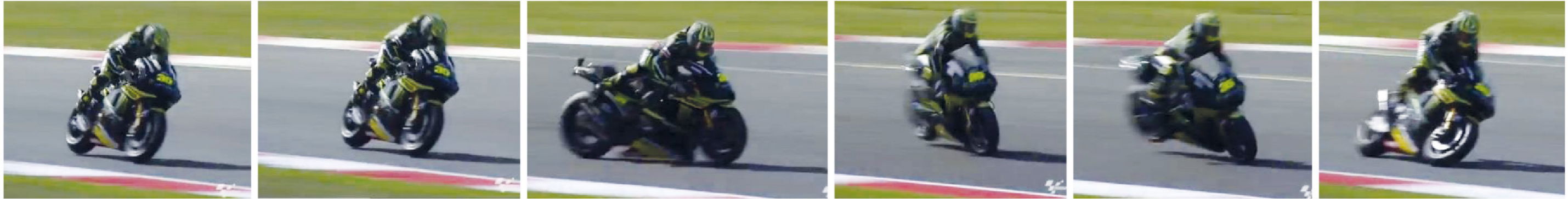
Figure 1: Development of a weaving movement at high speeds
